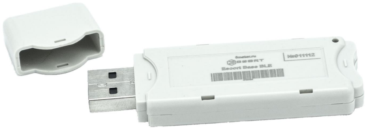
Fig. 3.3 Wireless capacitive fuel level sensor BLE-BASE-USB configuration tool design
